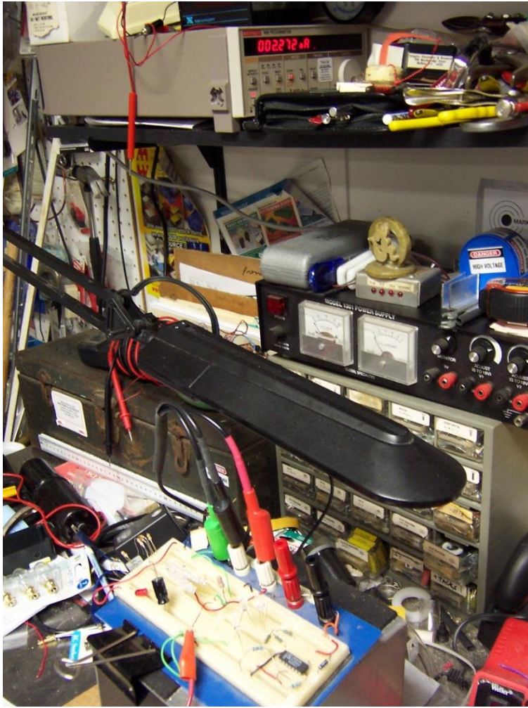
Keithley 486 Picoammeter reads 2.27 nanoamps constant current with or w/o resistor in series
